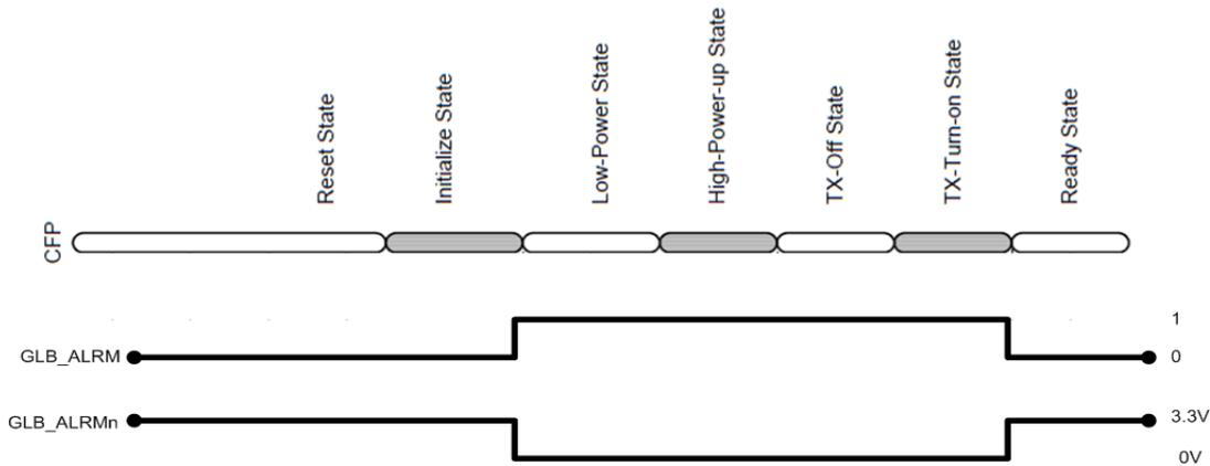
GLB\_ALARM is de-asserted during Reset and Initialize state, it is asserted in Low-Power, High-Power-up, TX-Off and TX-Turn-on states, then de-asserted again when Ready state is reached. GLB\_ALRMn is the hardware pin, and is the inverse of GLB\_ALARM.
